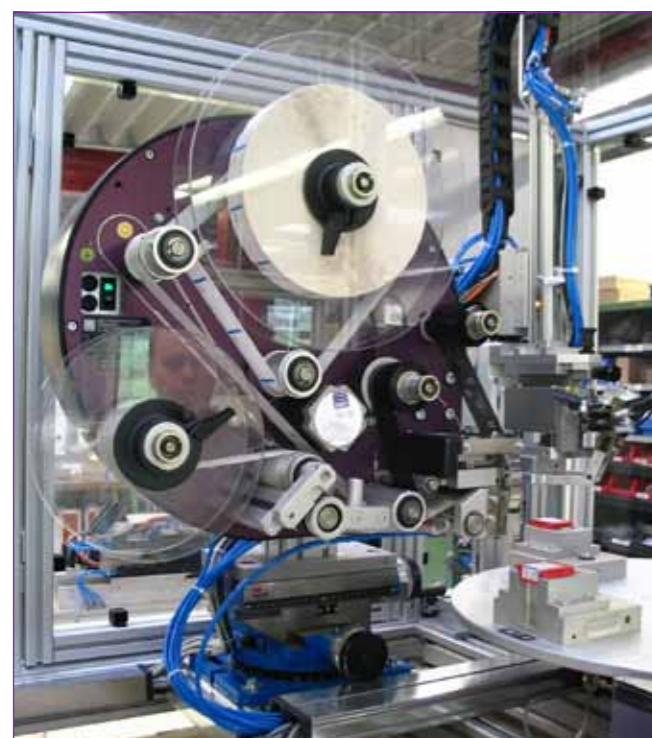
Label printed by thermal transfer method, centred and applied
