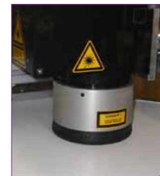
Laser protection enclosure in accordance with Laser Safety Class 1
