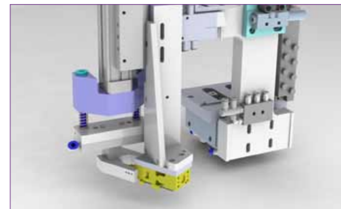
Label centering mechanism – gripping jaws closed
