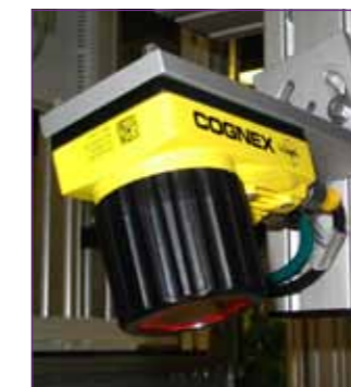
Camera system for reading the directly lasered Data Matrix code
